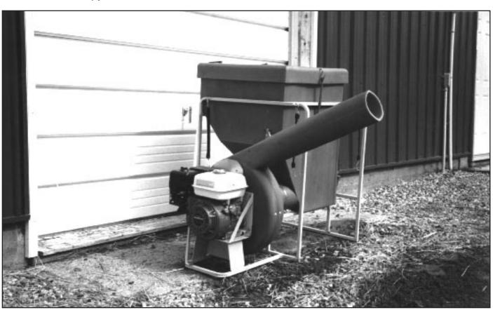
(fig. II.19–1), measure swath width while the spreader is actually mounted on the vehicle and preferably under the same conditions that you will experience during bait applications. Swath width measurement and actual bait applications should be done by traveling directly into or against the prevailing wind.
